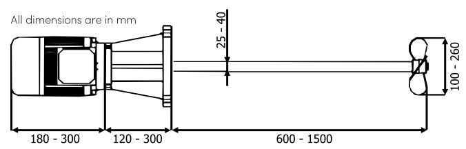
AGV Mixers are designed for use with a wide range of tanks with a variety of sizes (shaft lengths of 600 to 1500 mm). With either single or three phase motors and a choice of shaft material, the AGV mixers are suitable for any dosing system which requires a high-speed mixer. The AGV range feature a support flange as standard for tank mounting, allowing for ease of installation.
