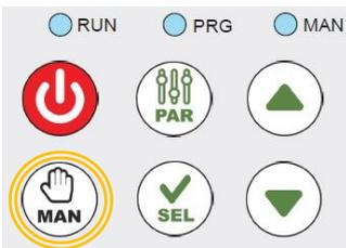
Pressing the **MAN** key switches to manual control, which allows the flow rate value (l/h) to be set with the two arrows.
