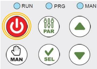
Press **RUN** to start/pause device. When restarting after each shutdown, the device will be in the last state it was left in (manual or automatic mode, in RUN or STOP). Instead of pressing **RUN**, functions can also be operated by external control. See chapter 6 for connection
