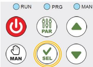
The **SEL** key to confirm parameter changes and to change numeric field during settings.
