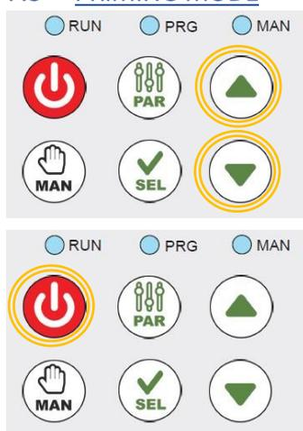
To enter this mode, with the system stopped, press the up and down arrow keys simultaneously for more than 5 seconds.
