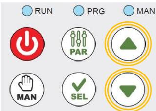
The arrow keys change values within the various parameters and can initiate the PRIMING function.
