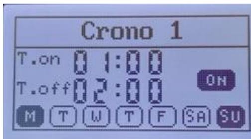
Once the CHRONO function is enabled, the inverter will switch on and off at the set times.
