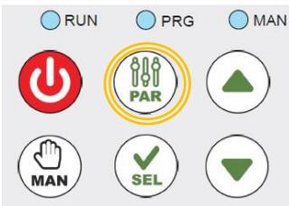
Press and hold **PAR** to access the parameter menu: Display Menu, Setup Menu, User Menu, Clock Menu and Chrono Menu. If no button is pressed, the system returns to the operational display after 25 seconds from the settings menu and after 45 seconds from the parameter menu.
