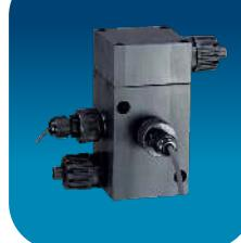
Outflow electrode for the detection of turbidity, operating according to the method NTU by a photodiode which reveals the quantity of reflected light, range 0-1000 NTU, maximum pressure 1 bar, recommended constant flow 1-15 l/h, PVC body, 1/2" nipple connector - tube with diameter 10x14 mm
