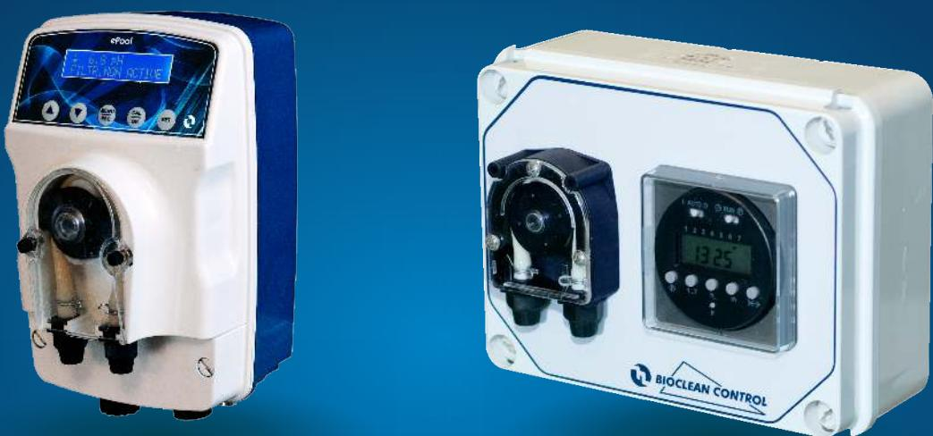
Etatron Peristaltic Pumps are designed for use with Dosing Systems with low flow rates and pressure. These pumps operate on the suction-compression created by rotors on a Silicone or Santoprene® tube, commonly used for simple dosing application, water treatment and laundry systems. Lightweight, and compact Etatron's Peristaltic Pumps are suitable for a wide range of Systems.
