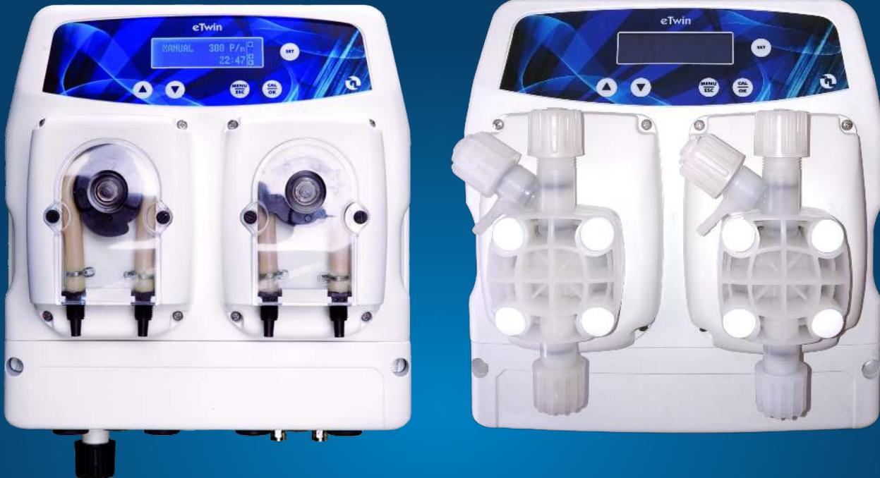
The eTwin is a compact, easy-to-use device which combines two dosing pumps and two parameters controllers designed to measure pH, Redox, Chlorine and the temperature. Designed with wet leisure and light-industry in mind, these dosing pumps are available in both peristaltic and solenoid versions.
