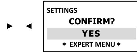
By confirming **YES**, the display goes out for about 1 second, then goes back to the **MEASUREMENT DISPLAY**
