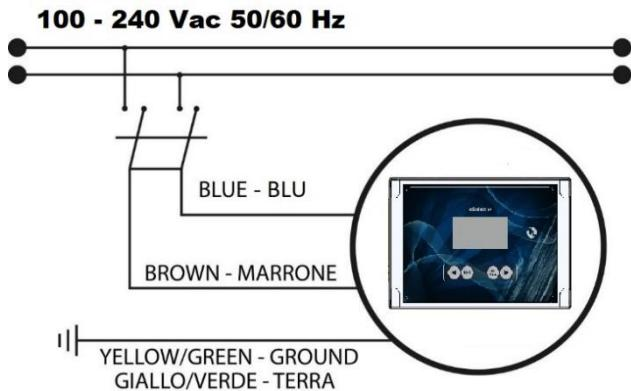
Fig. 1 – Electrical connection
