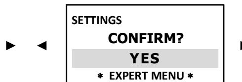
By confirming **YES**, the display goes out for about 1 second, then goes back to the **MEASUREMENT DISPLAY**
