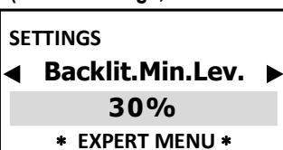
Adjusts display backlighting obtaining energy savings;
