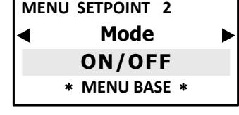
Direct mode: the output is active when the measured value is **lower** than the one selected in the setpoint, the metering pump injects Chlorine.
