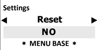
**DATA RESET:** resets default factory settings. ONLY to be used when the parameters do not match or if there are programming issues or when the operator wishes to restart from scratch. **NOT** to be overused as many resets may undermine the instrument's efficiency.
