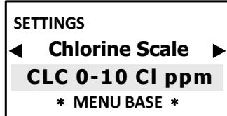
**IMPORTANT:** after selecting the **CHLORINE SCALE**, ENSURE the appropriate CHLORINE sensor is connected.
