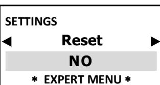
**DATA RESET:** resets default factory settings. ONLY to be used when the parameters do not match or there are programming issues or when the operator wishes to restart from scratch. **NOT** to be overused as many resets may undermine the instrument's efficiency.
