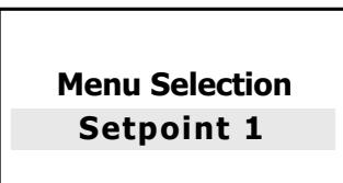
The instrument is preset by default for a 0 to 2 ppm range. By selecting the required chlorine range, the values and displays change accordingly. The setpoints will activate the output relays for the metering pumps or other devices once the setpoint level is selected.
