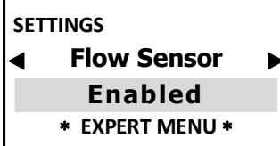
**Flow Sensor:** if there is no water flow in the probe socket (and possibly in the system), the flow sensor (proximity sensor), ENABLED, disables all outputs ensuring no chemical substance is added (DISABLED by default).
