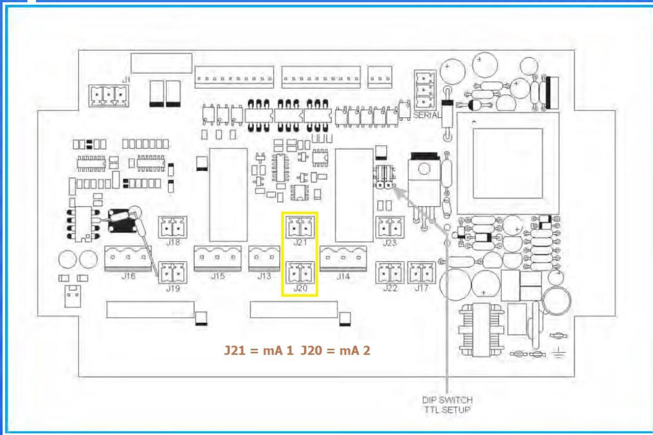
If using 4-20mA output pump should be connected to J21
