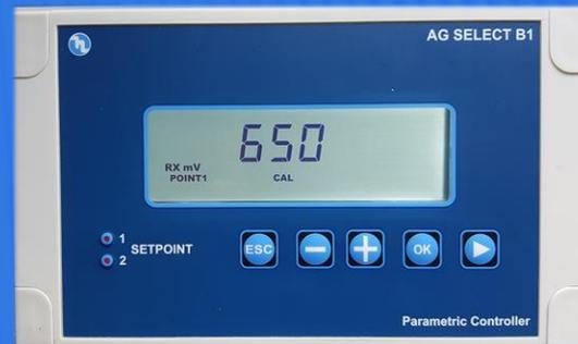
Place clean mV electrode into the buffer solution, mix slowly and then wait until display stabilises after around 1 minute. Use the PLUS and MINUS buttons to trim the reading to mV 650
