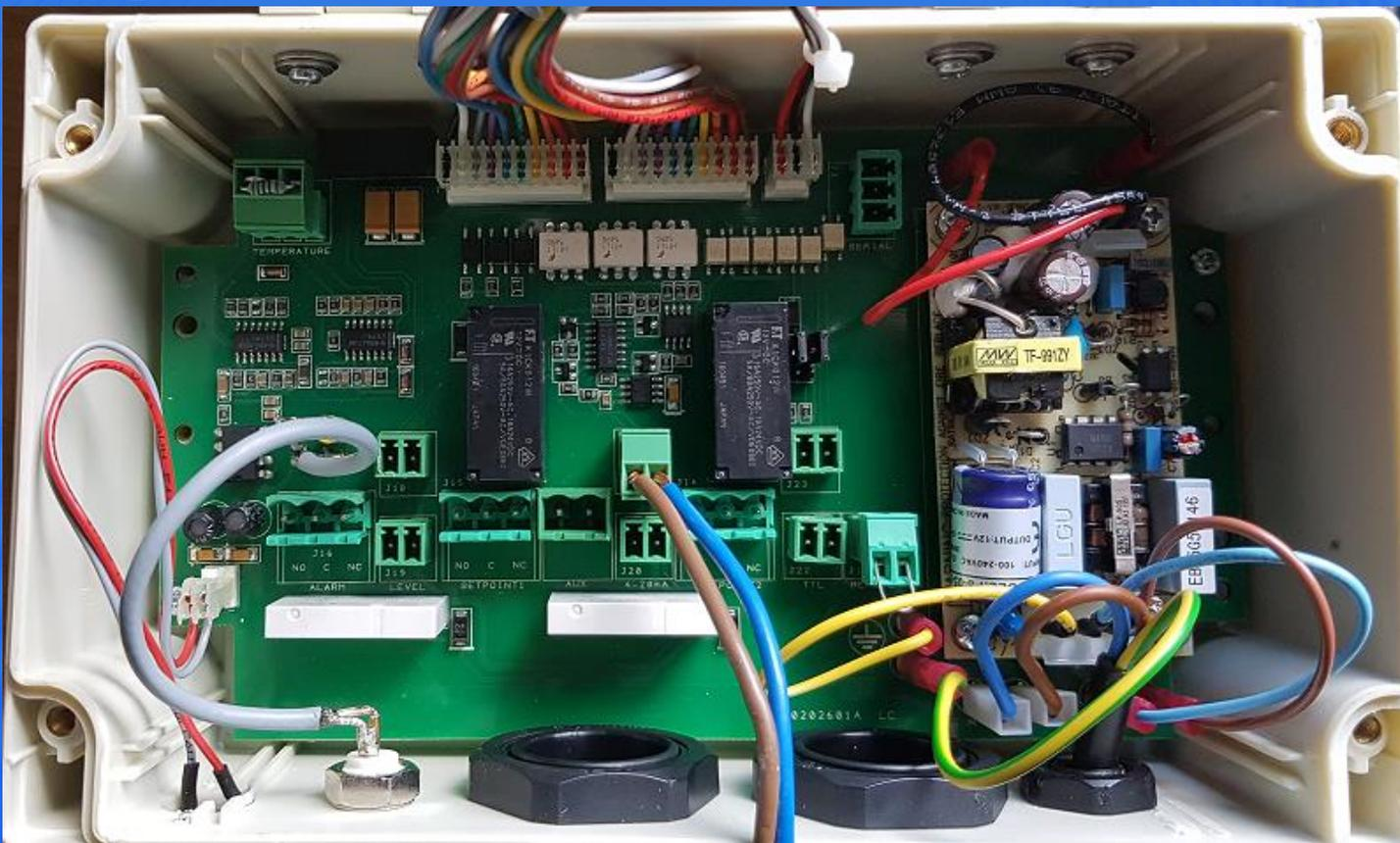
If using 4-20mA output pump should be connected to J21 as shown above
