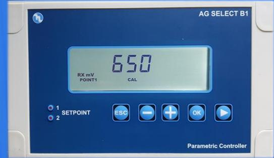
Place clean mV electrode into the buffer solution, mix slowly and then wait until display stabilises after around 1 minute. Use the PLUS and MINUS buttons to trim the reading to mV 650
