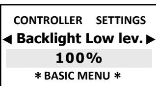
It adjusts the display save energy mode backlight level; touching any button will restore full 100% display operative brightness.
