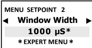
**Window Width (example with range 20000 µS):** pulses are timed ON and OFF according to the distance from selected set point, programmable, example: if selected set point is 700 µS EC and measured value is 600 µS, PWM mode will start after reaching 650 µS with Time/Pause pulses and decreasing the active time while reaching set point value. **\*Value shown according to selected K range.**
