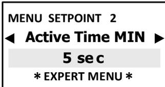
**Active Time MIN (minimum, programmable):** it sets the minimum time in which PWM is active, it overrules the minimum setting programmed, In case user has selected **Active time min 5 sec.**, this will be minimum time of PWM (check page 15, Timed Pulses function).
