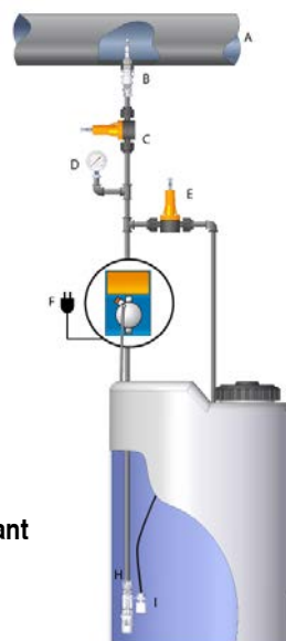
Fig.5 – Bleed operation for priming
