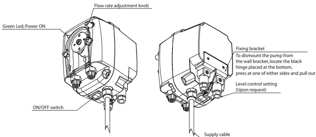
**NOTE:** if the dosing pump is supplied with level control setting (probe and floating switch not included), when the additive level is low, the green power LED turn yellow and the pump stops.
