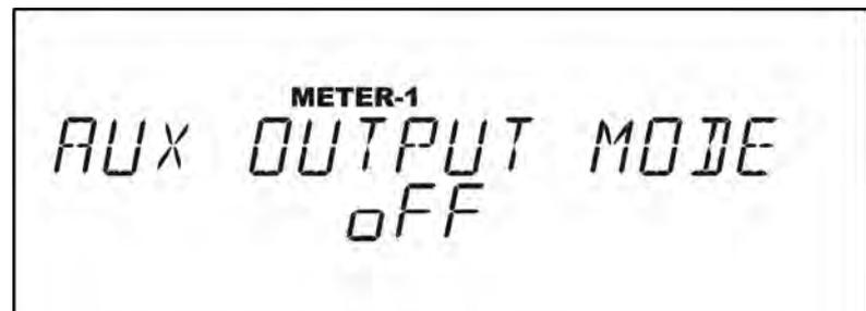
Once one of the two functions is activated (flocculant or cleaning) it is necessary to set the auxiliary outputs that need to be activated.
