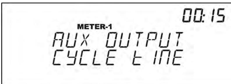
In the case of the **Flocculant** function it is possible to set hours and minutes of activation of the auxiliary output; the message appearing on the display is as follow:
